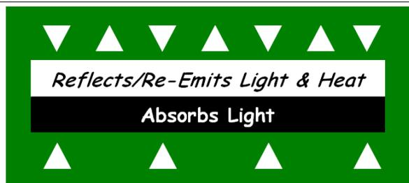
This arrangement is *far* easier to construct than other Casimir Force Devices since we are not dealing with nano-scale *structures*. We merely have to identify or create two materials, one which does an especially good job of absorbing EUV wavelengths and a second material that does an especially good job of reflecting these wavelengths. Preferably in the 50 nm wavelength or smaller. Smaller is *much* better!!!
