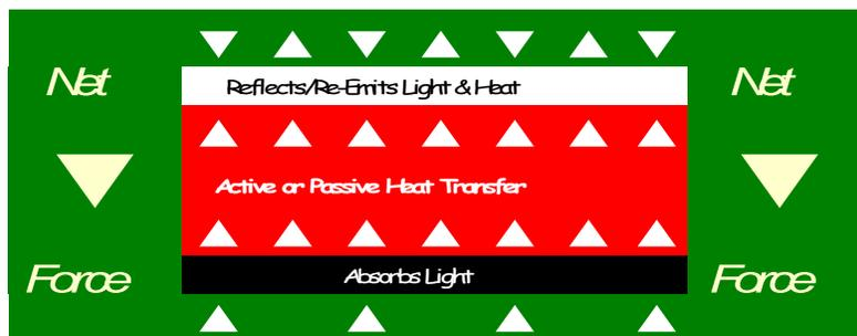
In other instances it is desirable to **actively** heat the reflective/emissive side using electrical, chemical, radiant energy or other method to *raise* its Black-Body-Radiation to *reflect/re-emit* more energetic wavelengths. In one embodiment, we can use high-temperature plasmas as the
