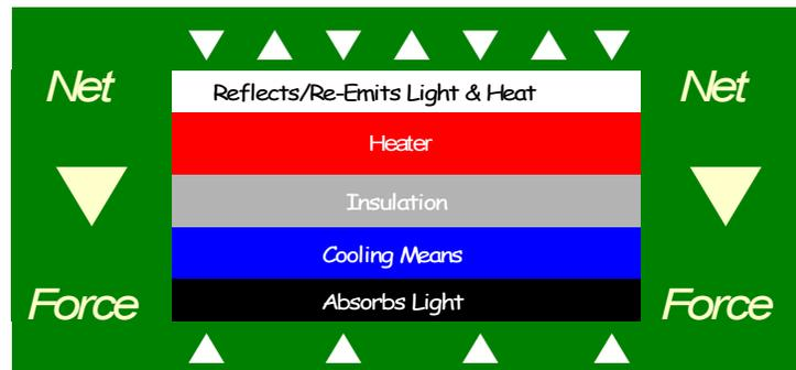
Proper textures can be combined *along* with various combinations of *different* materials to achieve the same basic results. Alternatively, as shown below, a single material with two textures, a light absorbing texture on one side and a reflective/emissive texture on the other side can be used as the two opposite surfaces. One advantage of this arrangement is that the reflective/emissive side can easily dissipate the heat that is generated in the absorptive side since both can be made of metal.
